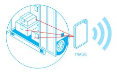
Pallets, storage boxes and / or ready-to-ship packages stored in the transportation fleet will be installed using TRAGG tools. TRAGG is a device with Bluetooth low energy (BLE) technology which is equipped with a temperature sensor and an air humidity sensor.
