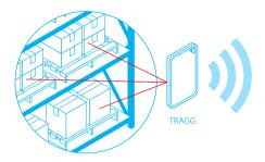
Pallets, storage boxes, and / or packages that are still stored in the warehouse will be installed using the TRAGG device. TRAGG is a device with Bluetooth low energy (BLE) technology which is equipped with a proximity sensor for easy tracking.
